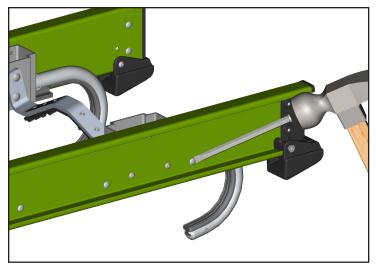
5. Use a hammer and chisel to remove any remaining rivet head material.
