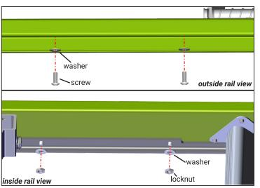
10. Using the new hardware provided, secure the new safety strip to the ladder as shown. Use a 3/8" wrench and 1/8" Allen wrench to tighten. Reapeat until all hardware is fastened.
