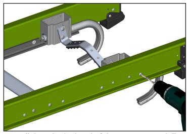
4. Drill thought the head of the rivet using a drill with 3/16" bit. Take care not to damage the fiberglass rail.
