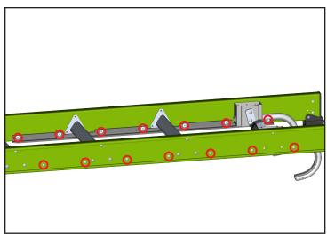
3. Identify the rivets to be removed.
