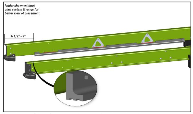
1. Take one of the safety strips and align the flat edge to the ladder as shown. The safety strip should start at 6 1/2" to 7" from the top of the end cap. Align the safety strip to run along the side of the rail using the rungs as guide. The safety strip will stick out a little as shown. Using a marker, mark the rail where the holes will be drilled. Repeat this step on both sides.
