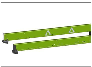
2. Using a 3/16" drill bit, drill through the rail at each marking. Take care not to damage the fiberglass rail. Go to step 9 on page 4 for final instructions.
