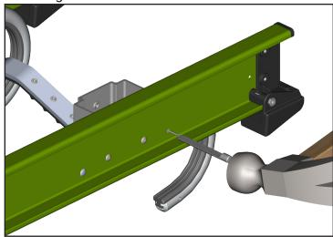
6. If needed, use a hammer and punch to remove rivet material left in the hole.
