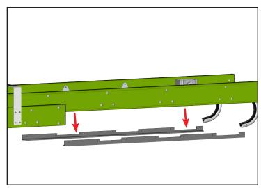
8. The existing safety strips can be removed and discarded along with any used hardware.
