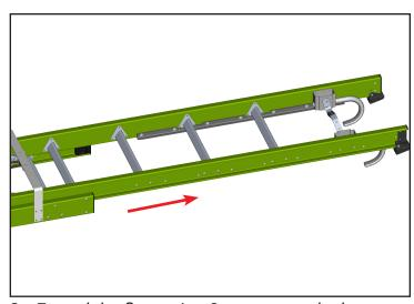
2. Extend the fly section 3 rungs past the base section.
