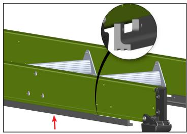
9. Align the flat edge of the new safety strip to the ladder as shown aligning the corresponding holes.
